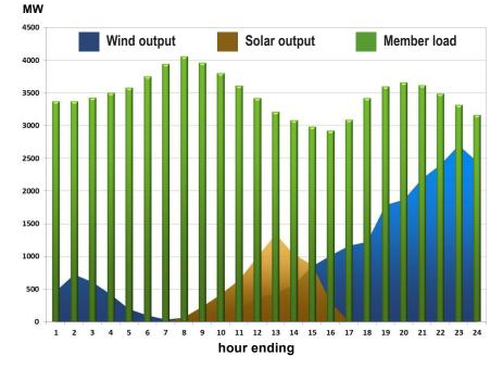
Information is based on actual hourly output from existing AECI wind generation and the Platte-Clay Solartech community solar project extrapolated to equal 5,000 megawatts of capacity.
